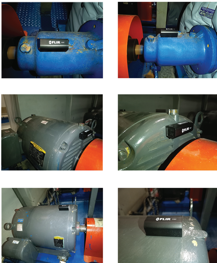
Figure 6.2 SV87 sensors shown mounted on machinery.
